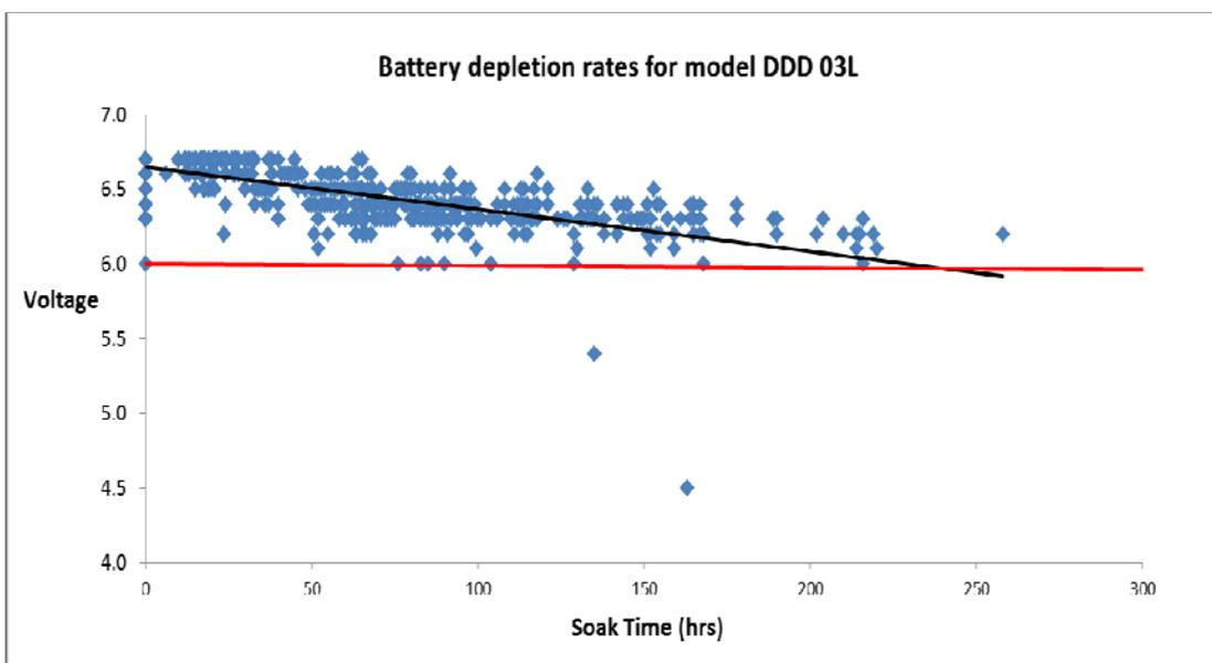
**Figure 6: Battery depletion rate for model DDD 03L**
