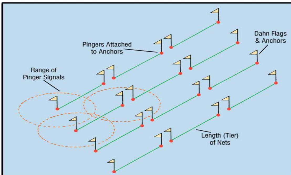
Figure 1: Schematic showing the industry suggestion for pinger deployment on static nets (courtesy of G.Caslake, Seafish)
