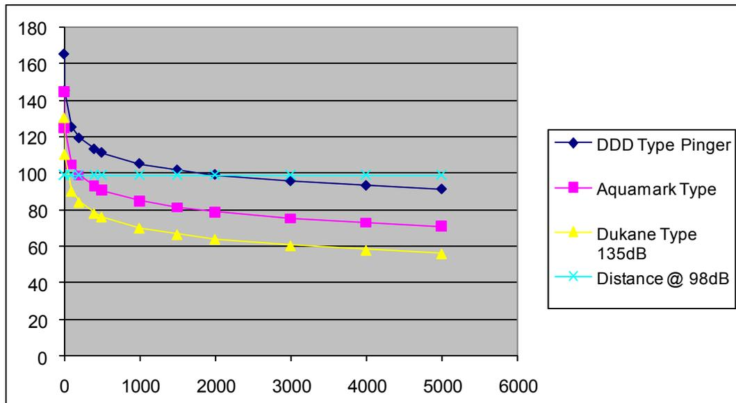
**Figure 2: Spherical spreading loss of acoustic signal with distance from source for three pinger types**
