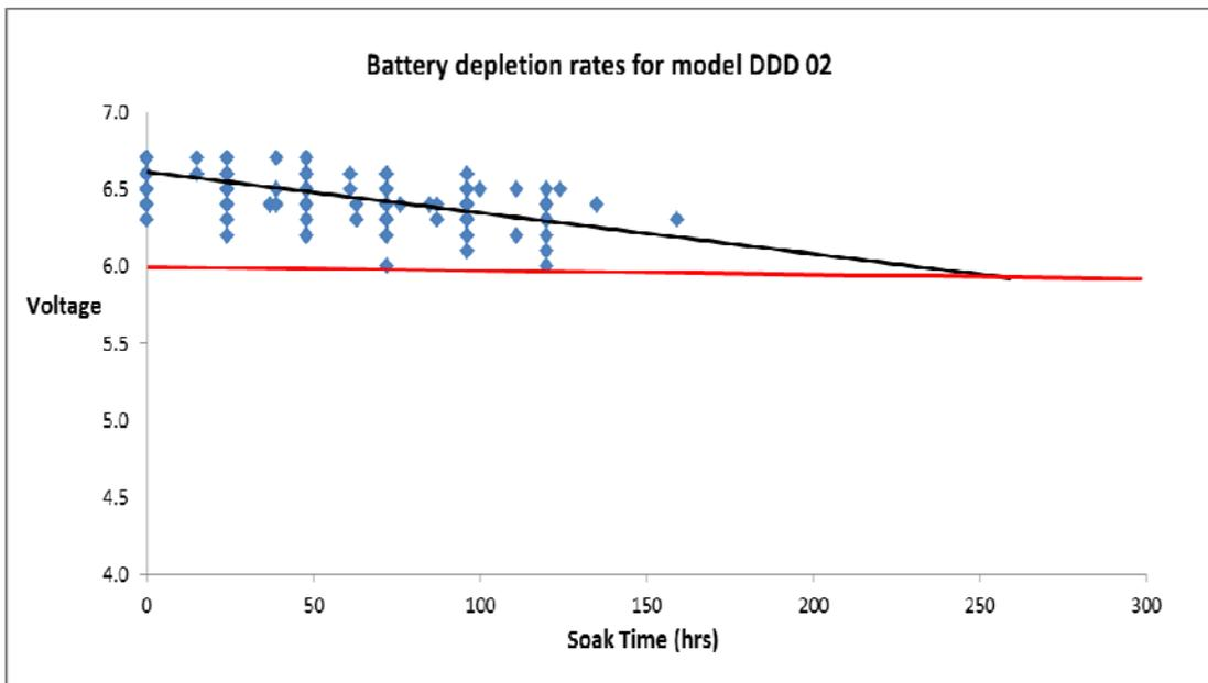
**Figure 5: Battery depletion rate for model DDD 02**
